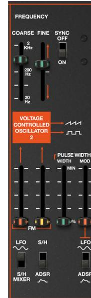
**FREQUENCY COARSE slider (green)** ..... [20(0.2)Hz...2K(20)Hz]
