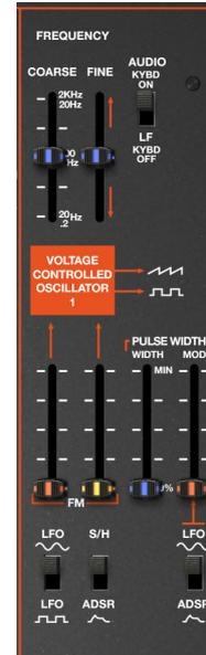
**FREQUENCY COARSE slider (blue).....[20(0.2)Hz...2K(20)Hz]**
