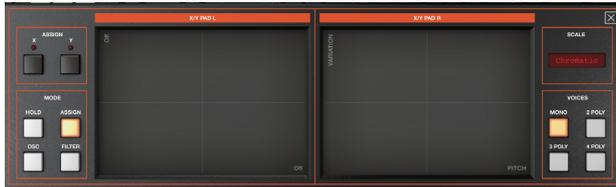
Drag across a pad to operate the parameters that are assigned to the X-axis (horizontal direction) and Y-axis (vertical direction). You can use this to play sounds or control parameters. For example, dragging horizontally on the right XY pad changes the pitch, and dragging vertically changes the note duration.
