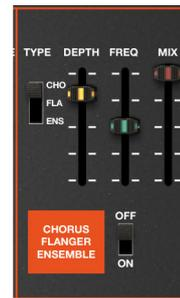
This effect gives the sound spaciousness and a sense of vibrato by combining the original sound with a signal whose pitch is modulated.
