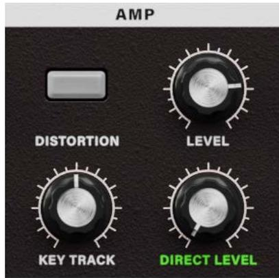
These parameters specify the volume. “LEVEL” specifies the volume of the internal sound source (OSC 1, NOISE) for the carrier. “KEY TRACK” adjusts how keyboard tracking will affect the volume, and “DISTORTION” specifies whether the sound will be distorted. The “DIRECT LEVEL” specifies the output volume level of the sound that is input from AUDIO IN.
