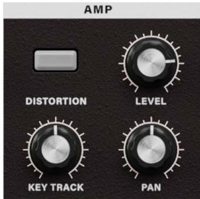
These parameters specify the volume. The sound that is created by passing through the oscillator and filter is amplified by the amp. “LEVEL” adjusts the volume. “KBD TRACK” adjusts how keyboard tracking will affect the volume, and “DISTORTION” specifies whether the sound will be distorted.
