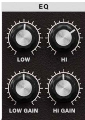
This is a two-band equalizer. Use EQ FREQ to specify the frequency that you want to adjust, and use EQ GAIN to adjust the gain of each frequency band.
