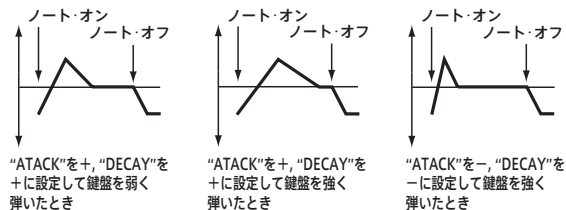
Pitch EG変化(タイム) (SOURCE=Velocity, INTENSITY=+の値)
