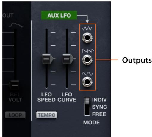
This addition to the vintage 2600 provides a CURVE slider, for continuous control of LFO shape, as well as a downward saw waveform.
