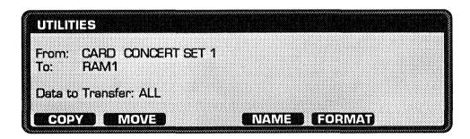
This page lets you quickly transfer complete sets of Performances, Patches, and Wave Sequences between cards and internal memory. (For transferring individual Performances and Patches, use WRITE.)
