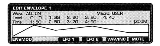
Since ENV 1 can be a modulation source for many of the Wavestation's parameters, EDIT ENVELOPE 1 is accessible through a number of pages. These include the EDIT AMP MOD, EDIT FILTER, EDIT LFO 1 (2), EDIT PAN, and EDIT PITCH pages under PATCH MACROS, and the EDIT MIX MOD page under WAVES.
