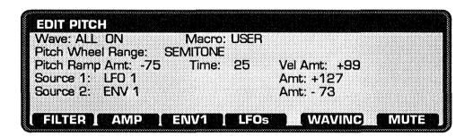
The Pitch module controls the frequency modulation of the Patch waves.
