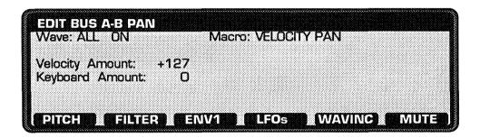
This page sets the modulation of the Pan position, the left-right orientation of the sound within the stereo field. Pan may be modulated by velocity and keyboard position.
