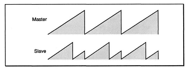
Since the overall timbre depends upon the pitch relationship between the slaves and the master oscillator, you can vary the timbre by modulating the pitch of the slaves. The pitch shift can be subtle (usually by LFO) or extreme (usually by envelope), as in the case of the classic "swept-sync" patch.
