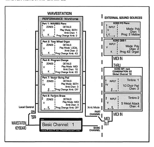
The figure shows the general features of the MIDI transmit section and an example of how someone might use the Wavestation as a master MIDI controller.
