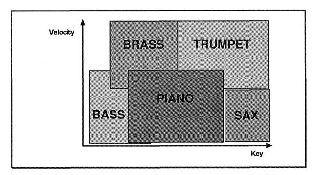
Assuming the Trumpet is Part 1 and the Bass is Part 5, setting up this example on the KEY AND VELOCITY ZONES page would produce a zone chart resembling this:
