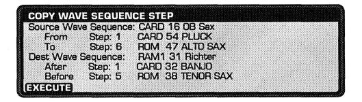
**NOTE:** During the copy operation, both the original and new versions of the destination wave sequence are remembered. The new version is temporarily stored in the available wave sequence step memory. To leave room for this, the number of steps that the destination will contain after the copy operation cannot exceed that of the available steps in the destination bank.
