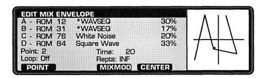
If the Patch is in 2 oscillator mode, the B-D axis (Y-AXIS) disappears. Waves A and C continue to be affected by the Mix Envelope.
