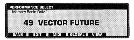
The PERFORMANCE SELECT page is the highest level of the Wavestation's menu system. It appears when you switch power on or after you press the EXIT switch a sufficient number of times.
