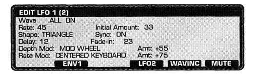
Since the LFOs can be modulation sources for so many of the Wavestation's parameters, EDIT LFO 1 (2) is accessible through a number of pages. These include the EDIT AMP ENVELOPE, EDIT AMP MOD, EDIT ENVELOPE 1, EDIT FILTER, EDIT PAN, and EDIT PITCH pages under PATCH MACROS, and the EDIT MIX MOD page under WAVES.
